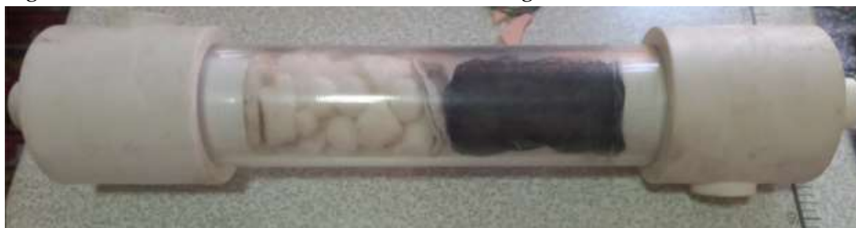
Figure 3. Overview of the water softener filter.
