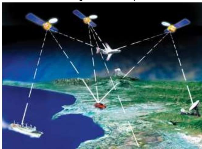
Figure 3. Communication of satellite system and GPS receiver.
