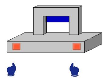
The lamp only comes on when the left switch and the right switch are closed. By combining their individual states, series-connected switches can be used as and gates.
